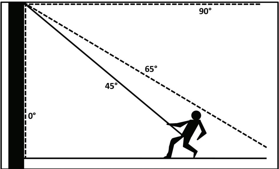
Pass on the information when the climber passes the point where any part of their work-positioning system is at 45° from the vertical.
